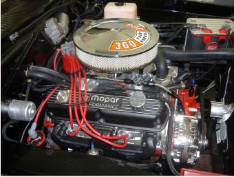
The cam is a Comp XE 284 flat tappet hyd. with roller rockers. The intake is an Edelbrock Performer RPM Air Gap that has been powder coated. The heads are also Edelbrock Performer RPM units. Fuel is supplied by a Quick Fuel SS 650 cfm double pumper with an electric choke. Spark is provided by a 6AL MSD unit and also includes the wires, coil and dist.
